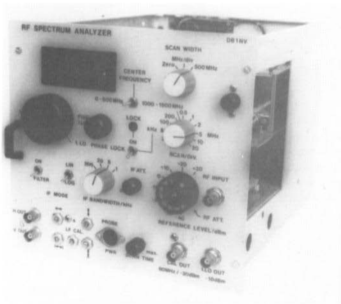
Fig. 9.1.: The author's spectrum analyser
